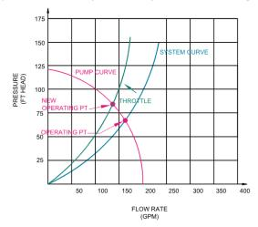
VFD: reduce flow by reducing frequency, which reduces RPM and the power of the motor. RPM changes so pump curve changes, parallel to the old curve.
