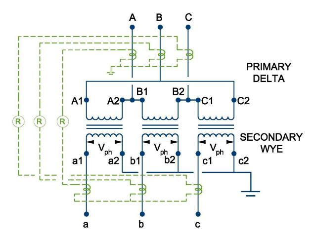
The correct answer is most nearly, (B) The relays on the wye side should follow a delta arrangement. The relays need to be arranged to account for the phase shift and the root 3 factor.
