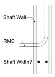
Based on NEC 2017, Table C.9, a maximum of fourteen 500 kcmil THHW wires are allowed in a trade size 6 RMC and ten wires are allowed in a trade size 5 RMC. Therefore, the RMC will be
